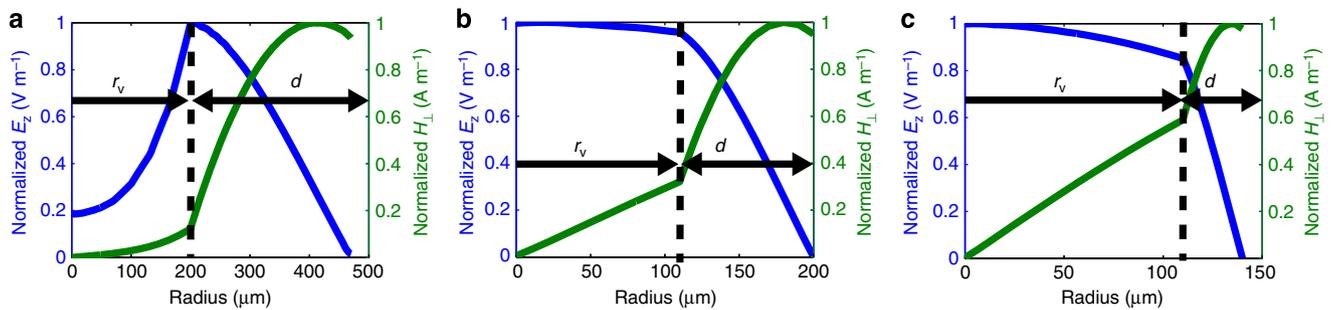
**Figure 6 | Electromagnetic field distribution.** The field distribution in the THz waveguide for (a) the non-relativistic design described in Fig. 4 with  $r_v = 200 \mu\text{m}$  and  $d = 270 \mu\text{m}$ , (b) the relativistic design in Fig. 5f for operation at 0.45 THz with  $r_v = 105 \mu\text{m}$  and  $d = 90 \mu\text{m}$  and (c) the relativistic design in Fig. 5f for operation at 1 THz with  $r_v = 105 \mu\text{m}$  and  $d = 30 \mu\text{m}$ .
