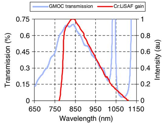
Fig. 2. Gain profile of the Cr:LiSAF crystal and the designed transmission spectrum of the GMOC.
